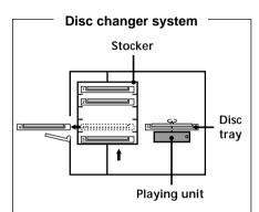
The disc changer consists of a playing unit, trays which hold the discs, and a stocker which transports the discs on their trays to the disc slot and the playing unit.
